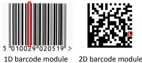
So . . . with the above definitions in mind, **PPM (Pixels Per Module) equates to how many pixels can be laid across each barcode module.** The Cognex Dataman Setup Tool outputs this value on screen, in a green text overlay (see image below). As a general guide line, Cognex readers & algorithms can read 1D barcodes down to about 1.0 PPM and read 2D codes down to 2.5 PPM\*\*.
