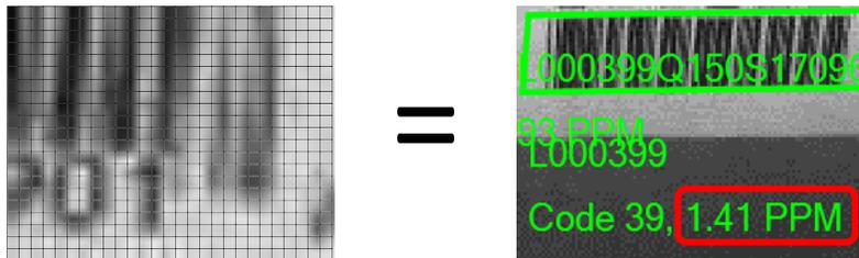
**What can affect PPM?** Camera/Barcode reader resolution, physical barcode module size (we usually measure in mils (1000’s of an inch), working distance, FOV & lensing.
